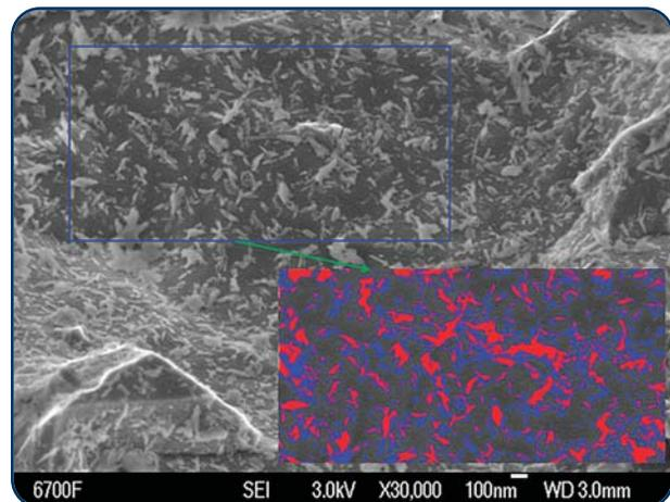
**Figure 2:** Phase Color-coding in Scandium Software Separates Out Nanometer-Scale-CaP Particles as Red-Blue Phase
