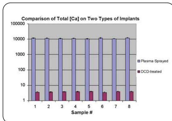
Figure 1: Comparison of total [Ca] on plasma sprayed and DCD-treated implants
