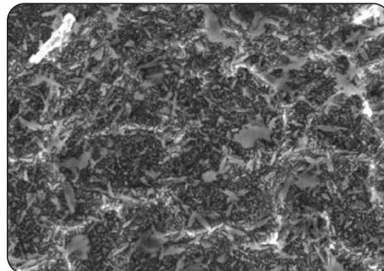
Figure 2: High Magnification FESEM Image of Implant Surface Showing Size and Shape of CaP Crystals
