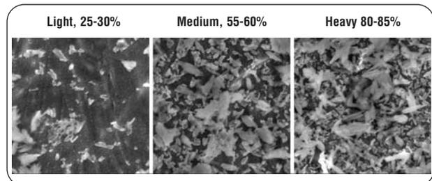
**Figure 1:** Field Emission SEM Images Showing Size, Shape and Distribution of Nanometer-Scale CaP Crystals with Light, Medium and Heavy Particle Coverages on DAE Surface (1  $\mu\text{m}$  x 1  $\mu\text{m}$  sample area at 30,000x)
