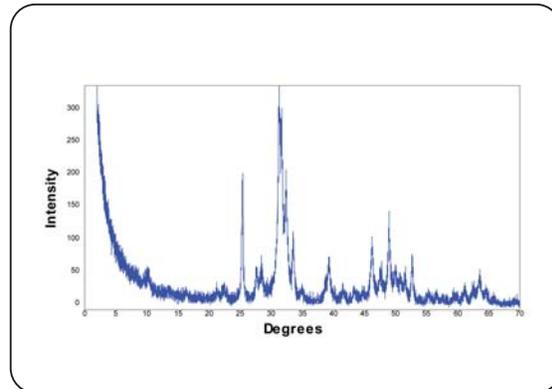
Figure 1: XRD Pattern For Dried CaP Powder Sample Which Shows It to be Purely Crystalline
