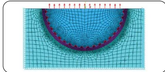
Figure 1: ANSYS model with meshing and uniformly distributed load pulling upwards.
