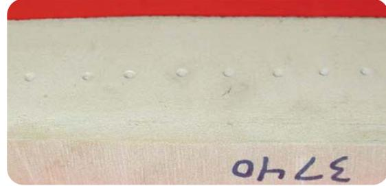
Figure 1: 3740 LAST-A-FOAM with eight (8) 3.25mm blind holes
