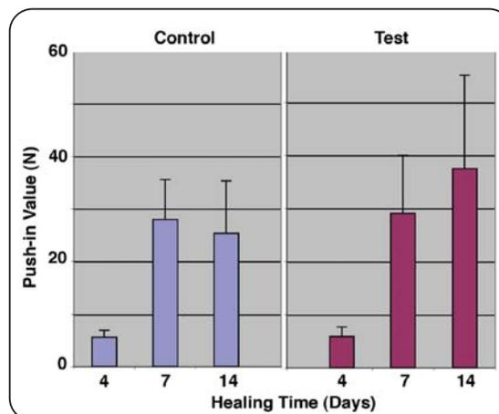
Figure 1: Implant push-in test in the rat femur model. All implants have the DAE surface. Test implant surfaces were additionally treated with DCD.
