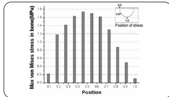
Figure 2: Stress distribution in bone at the failure (load = 44 KPa, E<sub>bone</sub> = 17 GPa)
