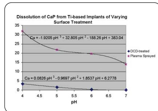
Figure 2: Dissolution trends of plasma sprayed and DCD-treated implants
