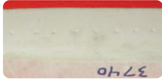
Figure 1: 3740 LAST-A-FOAM with eight (8) 3.25mm blind holes
