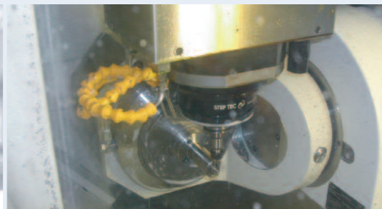
Fig. 8 Laboratory image of the CNC machine milling the definitive Encode Abutment.
