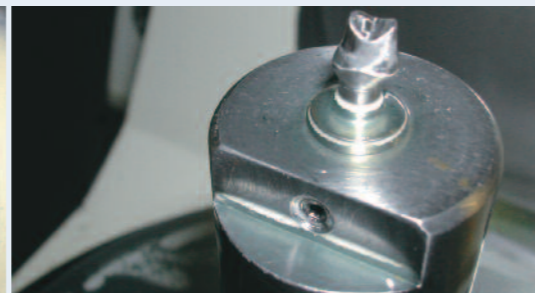
Fig. 9 Laboratory image of the definitive Encode Abutment just prior to removal from the milling unit.
